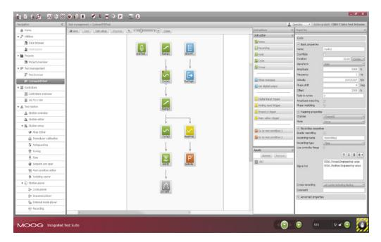
The Test Builder allows the user to quickly create and/ or edit test definitions.
