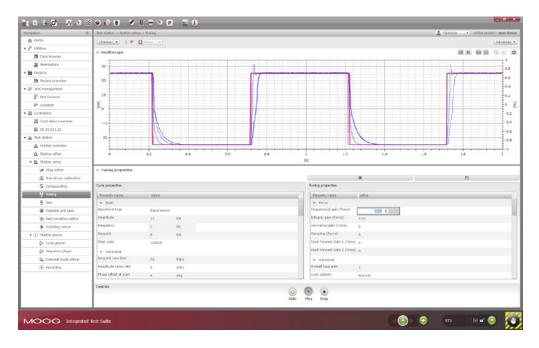
The Tuning screens in the Integrated Test Suite allow the user to set a command signal and view the response of the feedback signal in real time.
